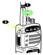
Figure 4-7 Verifying a Programmed Channel.
