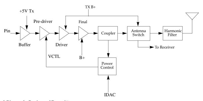
Block Diagram for Receiver and Transmitter
