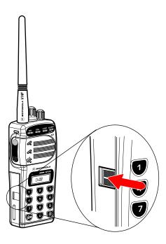
Figure 1-1 Slide Battery Latch
