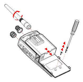
Figure 1-3 Remove Radio Chassis
