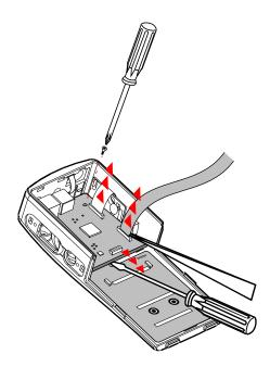
Figure 1-6 Remove Controller Board
