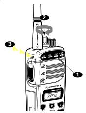
Figure 4-11 Selecting the Frequency Step Size.
