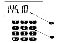
Figure 4-12 Using the Keypad to Select a Receive Frequency.
