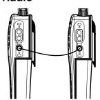
Figure 4-2 Cloning a Radio.
