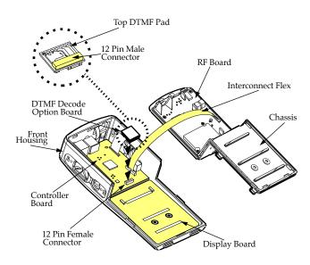
Figure 3-4. Exploded View of the Radio with DTMF Option Board
