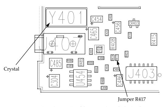
Figure 4-1 Location of the Jumper R417 on the GP68 Radio.
