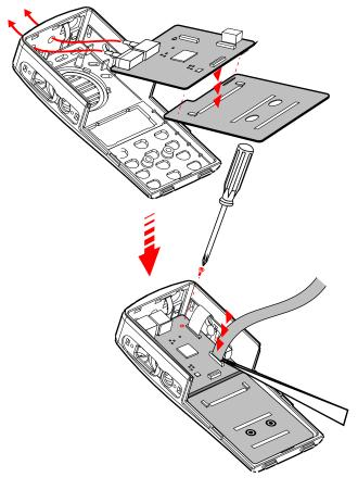
Figure 1-8 Replace Controller Board and Display Board
