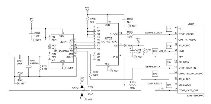
Schematic Diagram/Parts List for DTMF Decoder Option Board (PMLN4063)
