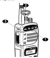
Figure 4-18 Selecting the Transmit PL/DPL Code.
