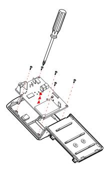
Figure 1-4 Remove RF Board
