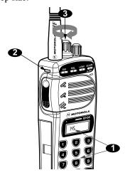
Figure 4-13 Using the Channel Selector Knob and Keypad to Select a Receive Frequency.
