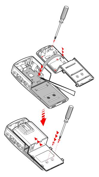
Figure 1-9 Replace Radio's Chassis
