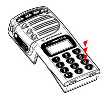
Figure 1-7 Remove Display Board
